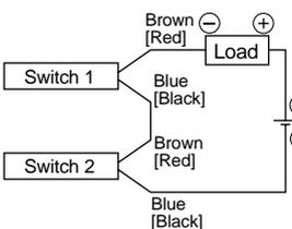
When 2 switches are connected in series, the load may malfunction because the load voltage will decline when in the ON state. The indicator lights will light up when both of the switches are in the ON state.
