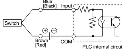
The connection method will vary depending on the PLC input specifications. Connect accordingly.
