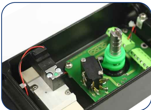
Solenoid valve and limit switches
